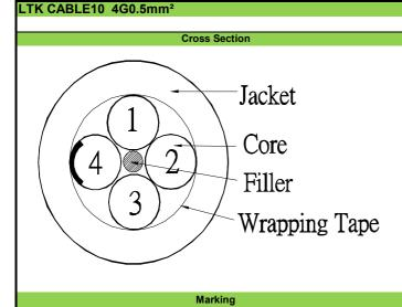
XXXXXXm MM/DD/YY LTK CABLE10 4G0.5 300/300V E148000**R** AWM STYLE 2464 80℃ 300V VW-1 -LF- PCxx CE RoHS conform
