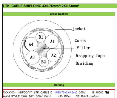
Description Rated Temperature (°C) -20~80°C Rated Voltage (V) 300V Flammability VW-1
