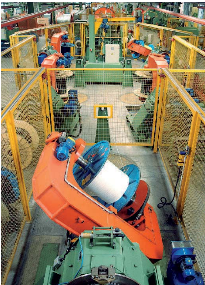
Large cabling machine with backtivist at our Windsbach factory.
